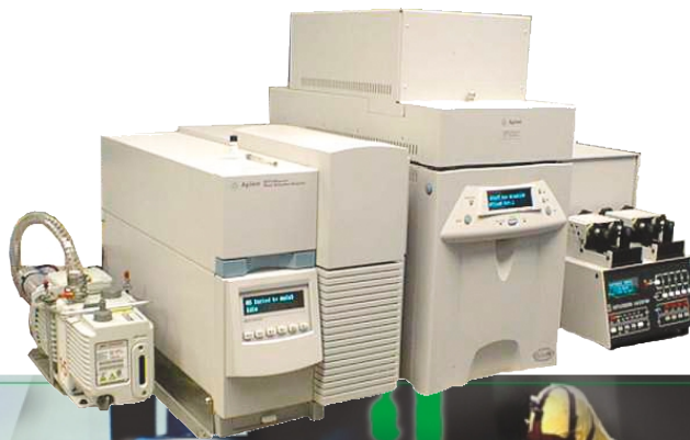
Agilent 6850 Gas Chromatograph and 5973N Mass Selective Detector used for the detection, identification and confirmation of chemical compounds.
